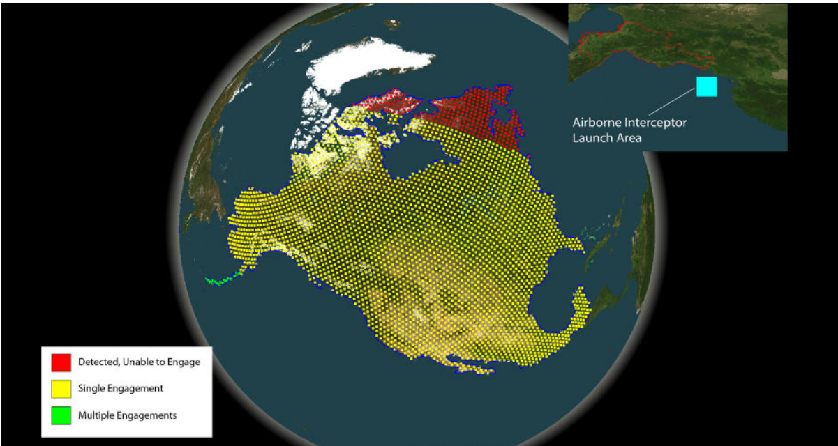
Figure 9B: Notional Defensive Coverage of North America from North Korean ICBM (4 km/s interceptor, 50-second engagement delay)
