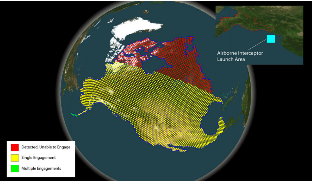
Figure 5A: Notional Defensive Coverage of North America from North Korean ICBM (4 km/s interceptor, 75-second engagement delay)
