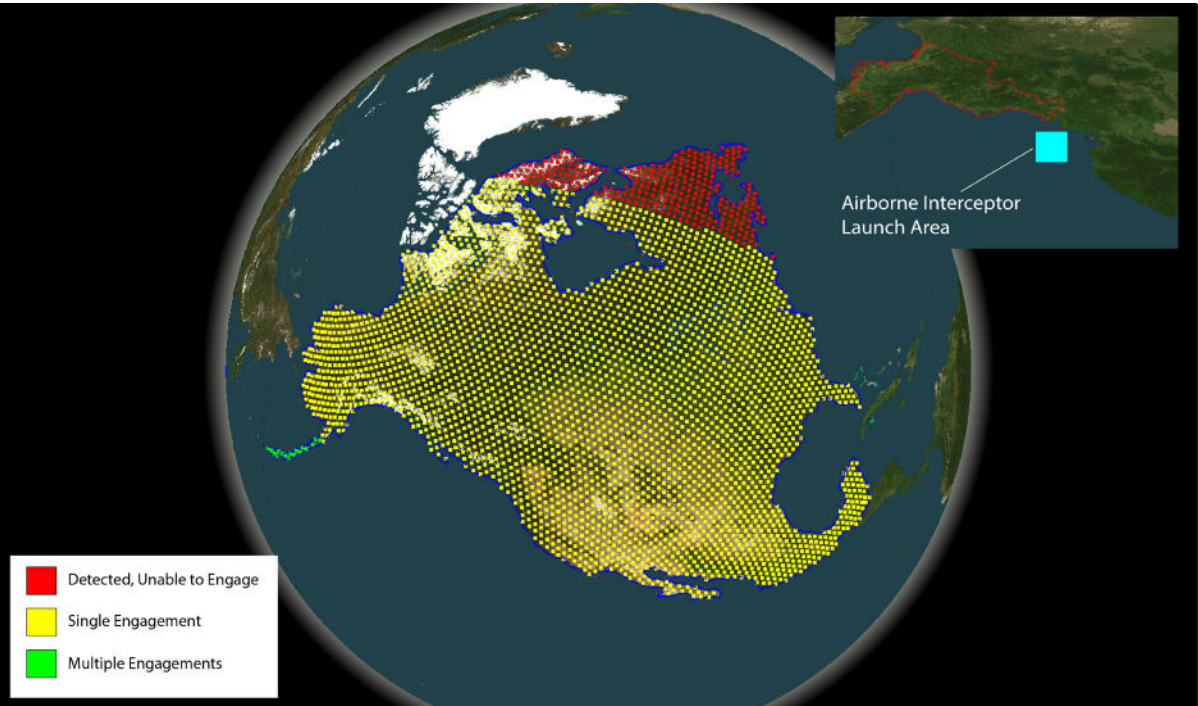
Figure 5B: Notional Defensive Coverage of North America from North Korean ICBM (4 km/s interceptor, 50-second engagement delay)
