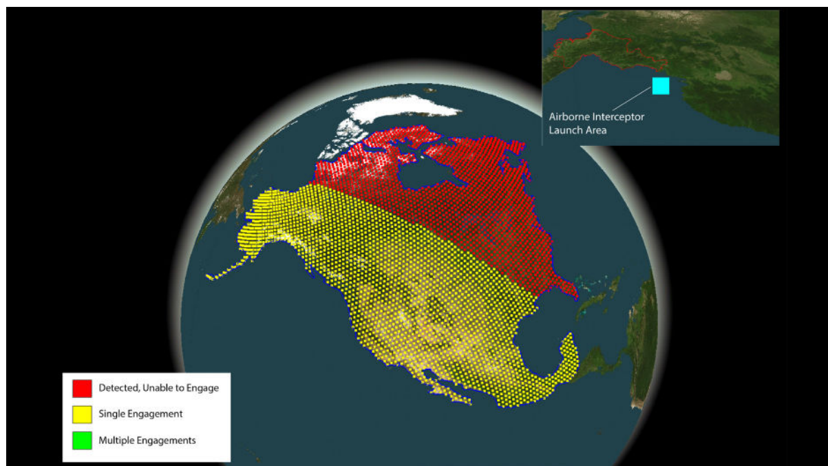
Figure 9A: Notional Defensive Coverage of North America from North Korean ICBM (3 km/s interceptor, 50-second engagement delay)
